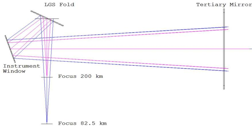
Fig 2 Telescope interface showing the focus position of the LGS at 82.5 km altitude and 200 km altitude.
