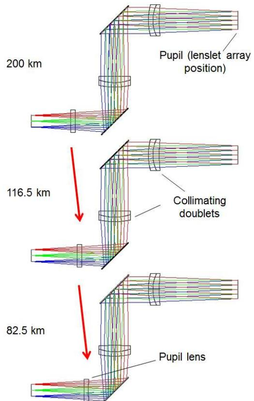
Fig 3 Optical layout of a single LTWS channel (200, 116.5 and 82.5 km).
