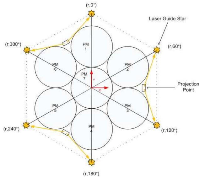
Fig 1 Relative position of the LGS with respect to the telescope coordinate system. The primary mirrors are also included as reference. The LGS are equally spaced around the z-axis at 60 degree intervals
