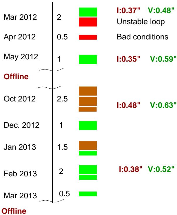
Fig. 2. Summary of SAM commissioning over the last year. The approximate number of nights used by each run is indicated. The nights are coded by the green color when a useful performance was achieved, by brown when SAM gave little gain in resolution, by red when the instrument was not operational. Median FWHM image quality in the *I* and *V* bands is indicated for some nights. Periods when the instrument was offline (shutdowns) are marked.
