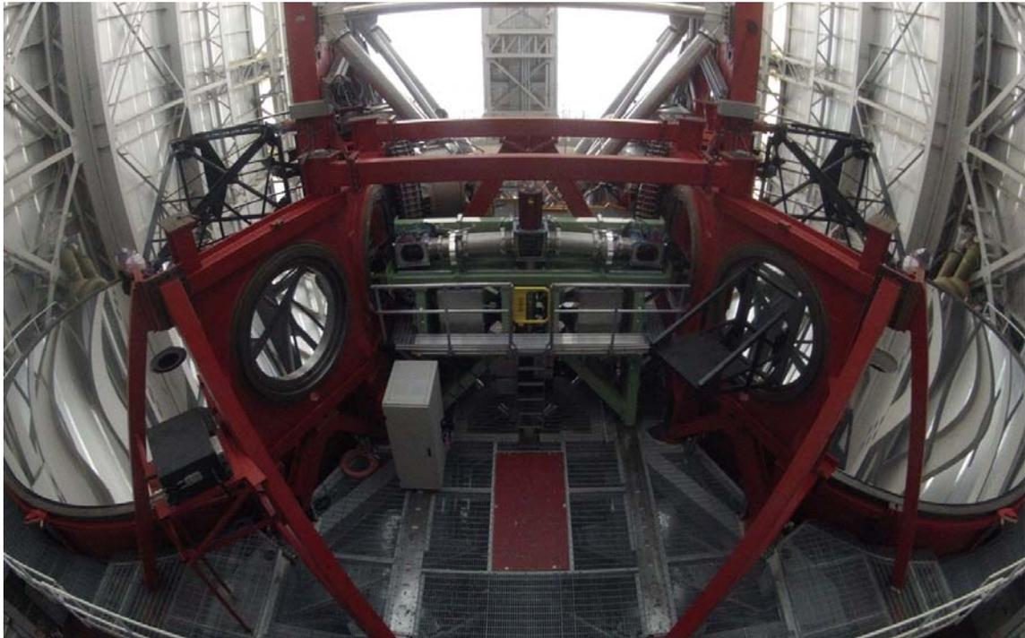
Figure 2 - A wide-angle view of the two 8.4 m primary mirrors of the LBT with the LBTI instrument mounted at the central focal stations. The red steel is the elevation structure of the telescope, and the green steel near the center is the support structure for the LBTI beam combiner and cameras.
