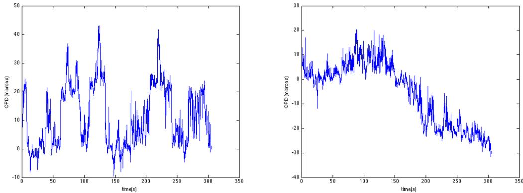
Figure 4 - These plots show the Optical Path Difference (OPD) between the two sides of LBT as measured by the dispersed fringes in LBTI/LMIRcam (see Figure 5). The first plot (left) has focus offloading turned on (accumulated focus on the adaptive shell is offloaded to hexapod piston) which creates noticeable jumps in OPD. The second plot (right) has focus offloading off (operated at very low gain) and the jumps in OPD have been suppressed into the atmospheric piston variations.
