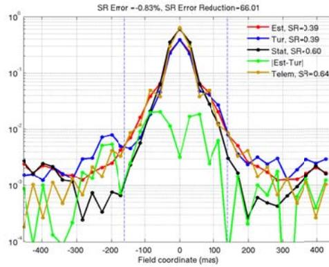
Figure 3 Red: TTR turbulence long exposure PSF estimate obtained from (3.10), Blue: truth obtained from left expression in (3.4), Black: static PSF obtained from right expression in (3.4), Green: absolute estimation error, Brown: telemetry long exposure PSF obtained from (3.9). Dashed vertical lines indicate the FoV of the turbulence data prior to OTF interpolation.
