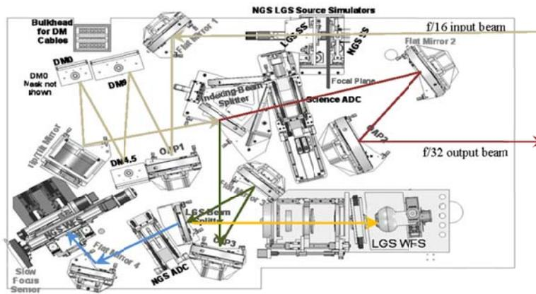
Figure 1 Schematic of the Gemini Canopus AO bench.
