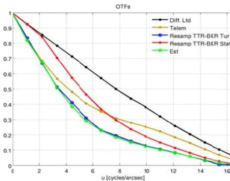
Figure 4 Black: diffraction limited OTF (denominator of (3.10)), Brown: telemetry OTF (3.9), Blue: turbulence OTF (left expression in (3.4)), Red: static OTF (right expression in (3.4)), Green: estimated turbulence OTF (3.10).
