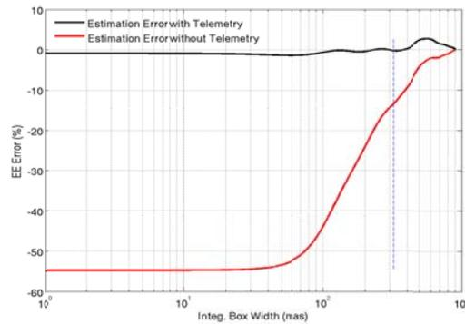
Figure 5 Black: EE estimation error for a PSF computed with WFS telemetry, Red: EE estimation error for a PSF computed without telemetry. The dashed vertical line indicates the FoV of the turbulence data prior to OTF interpolation.
