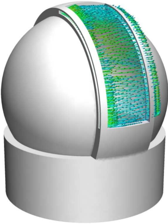
**Fig. 2.** A figure showing a model of the WHT dome with an air curtain placed across the dome aperture entrance.
