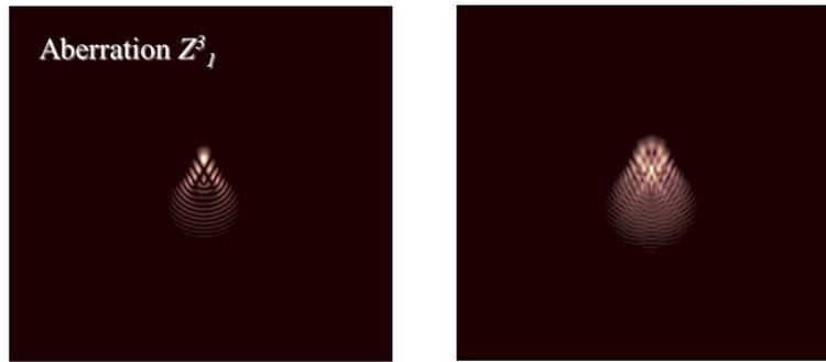
Fig. 11 Circular modulation on the pin of the simulated pyramid, for Zernike mode  $Z_1^3$ . Left: no modulation; right: modulation, with a 8-points sampling. This picture is used only for display purposes, since the average is done on the four re-imaged pupils, and not on the focal plane, to avoid interference patterns.
