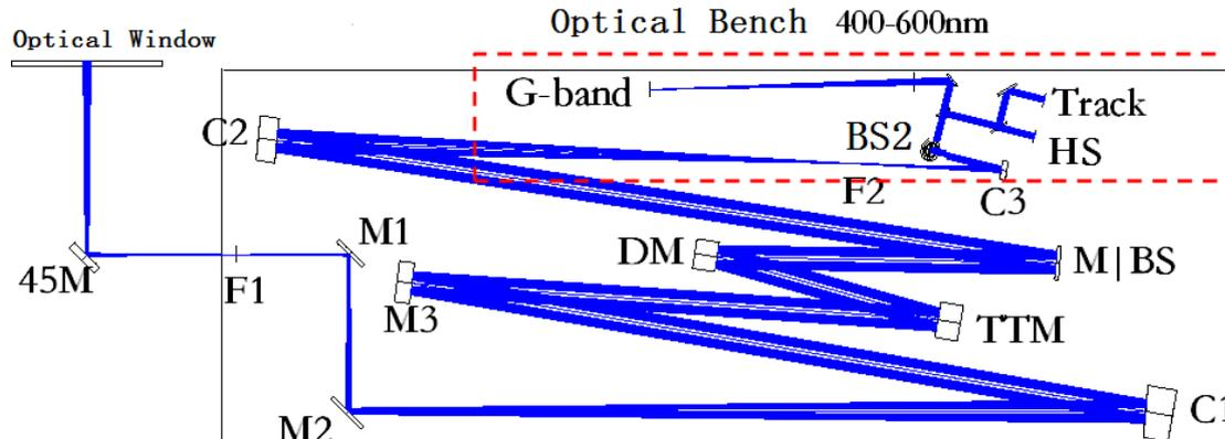
Fig. 4. The optical layout of the high-order AO system on top bench, two layers bench is obtained.
