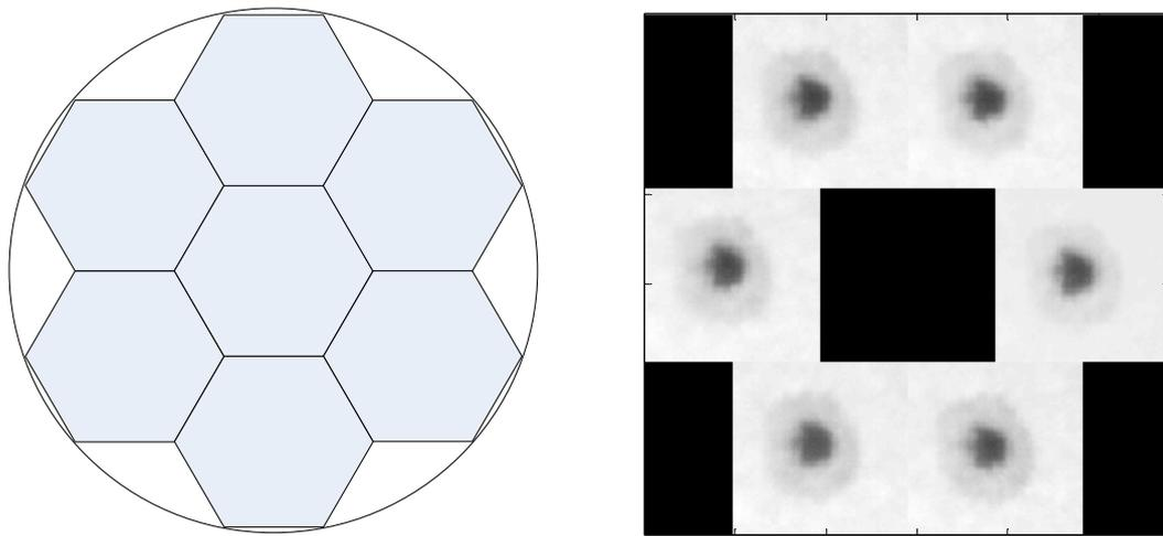
Fig. 6. Pupil and focus geometry of Large FOV SHWFS
