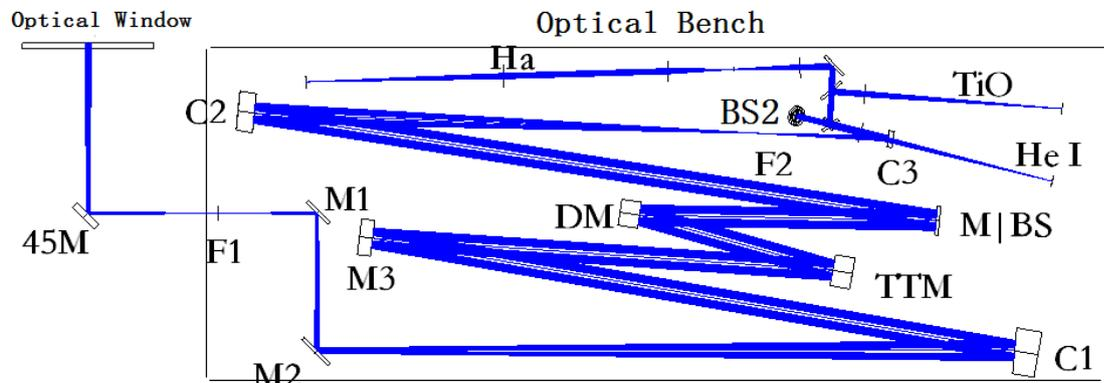
Fig. 5. The optical layout of the high-order AO system on low bench, two layers bench is obtained.
