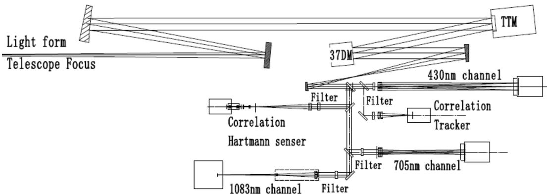
Fig. 2. The optical layout of the AO imaging system
