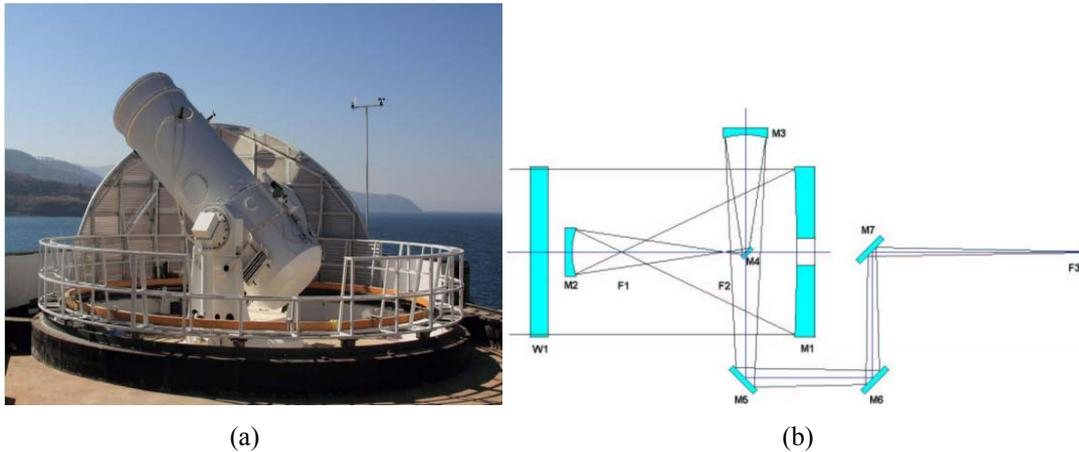
Fig. 1. New Vacuum Solar Telescope and its wind screen (a) and the optical diagram of NVST (b)
