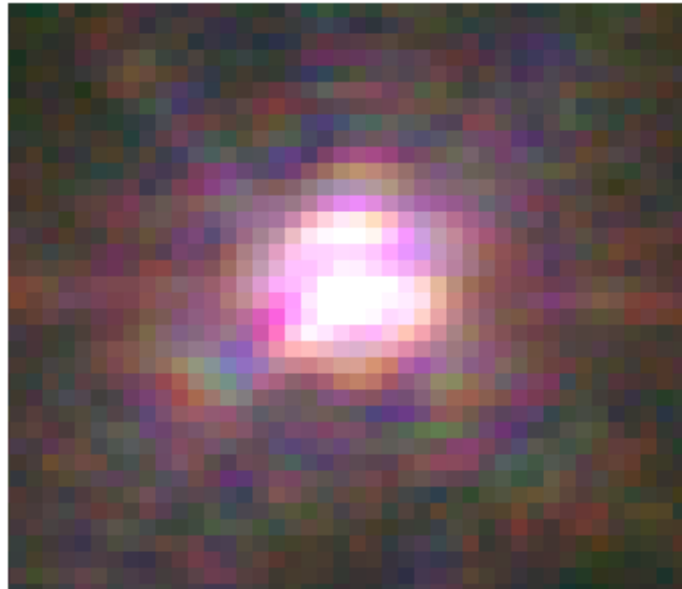
Fig. 3: Colour PSF reconstructed from three channels of the IFU datacube at 700, 850 and 1000nm. Each spaxel in this image is 16mas, and the FWHM of the PSF is about 50mas at 850nm. The chromatic effect caused by the diffraction pattern scaling with wavelength can be seen.
