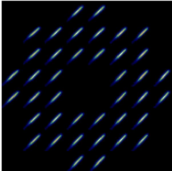
**Fig. 2.** An example of SH spot pattern, as it will be recorded on CANARY for the maximum off-axis angle.
