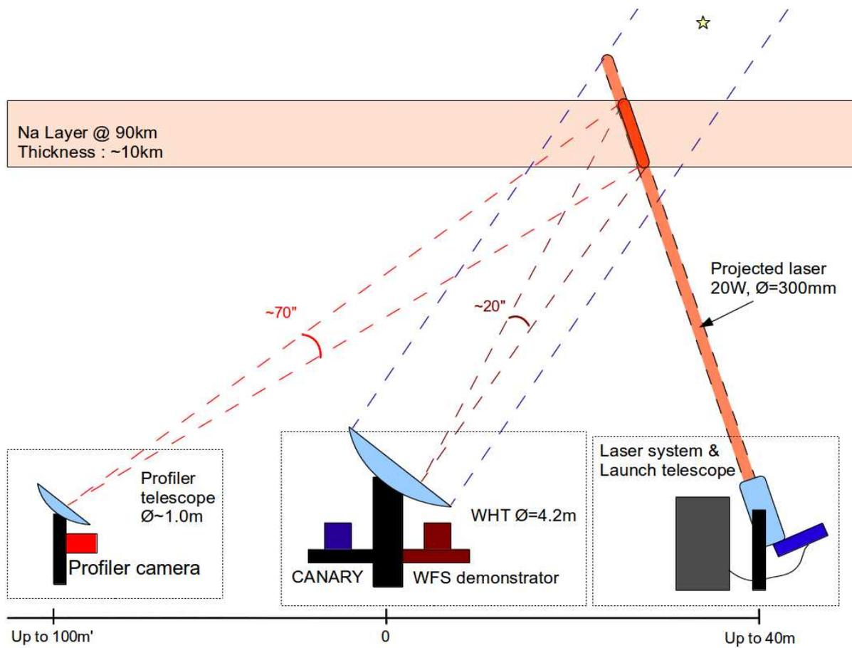
**Fig. 1.** The various components of the proposed experiment.
