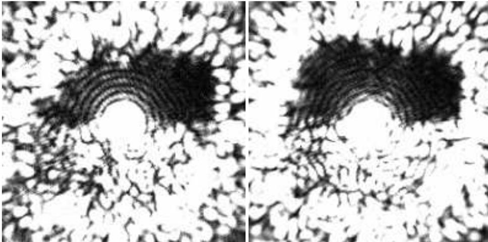
**Fig. 6.** Laboratory SCC images after aberration correction in polychromatic light ( $\sim 6\%$  bandwidth) using one (left) or two (right) reference channels.
