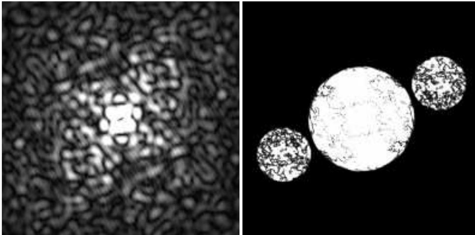
**Fig. 2.** SCC image in monochromatic light (left) and the modulus of its Fourier transform (right).
