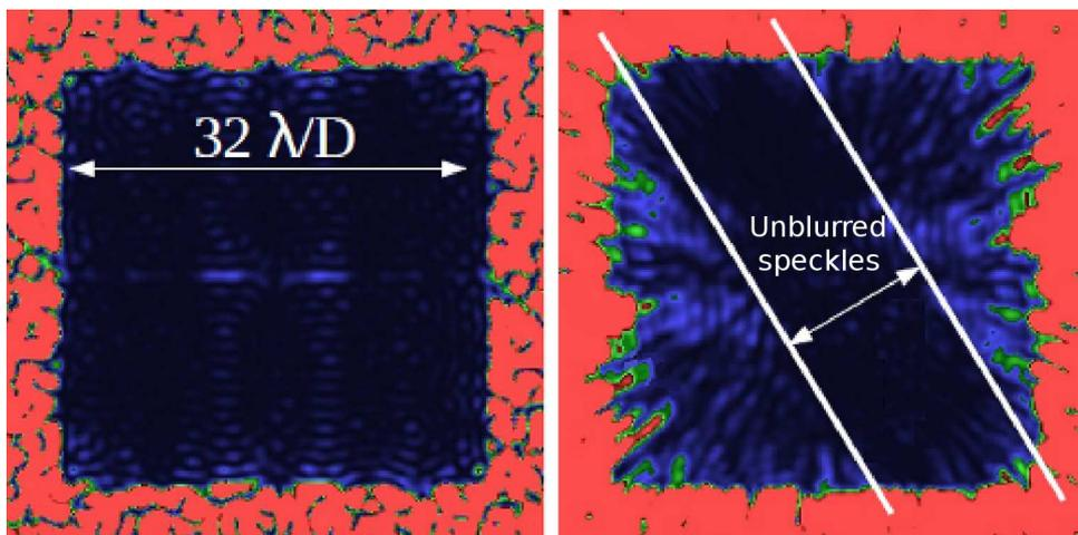
**Fig. 3.** Dark hole in the SCC image after aberration correction with a  $32 \times 32$  DM. Left: monochromatic light. Right: 10% bandpass. Numerical simulations with only phase aberrations.
