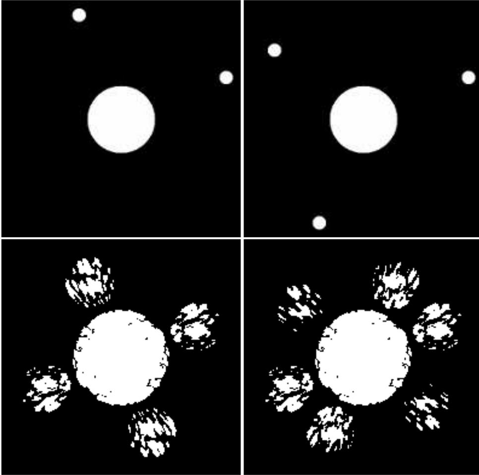
**Fig. 5.** SCC Lyot stop with two (left) and three (right) reference channels.
