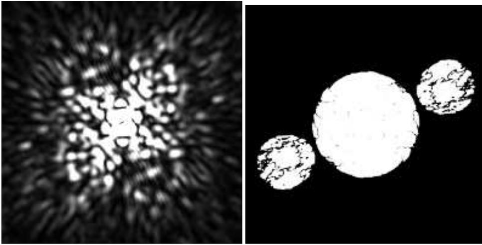
**Fig. 4.** SCC image for a 10% bandwidth (left) and the modulus of its Fourier transform (right).
