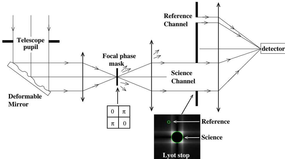
**Fig. 1.** Schematics of a self-coherent camera associated with a FQPM.
